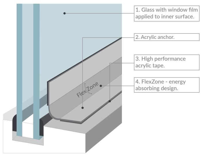
The OVAGLAS® Flexible Anchoring System is installed on all four sides of the window test specimens with adhesion to the powder coated aluminium frame and adhesion to the inner surface of the film.
